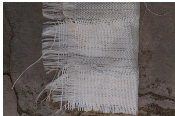
Fig3.2 Woven Glass filaments
