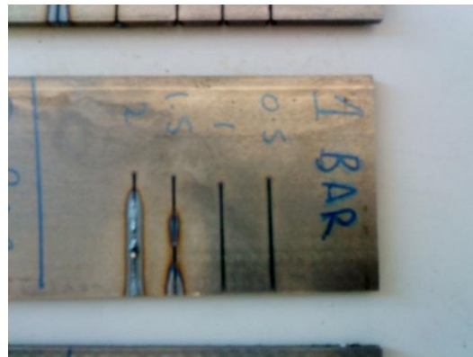
Figure 2: cut for 1 bar pressure
