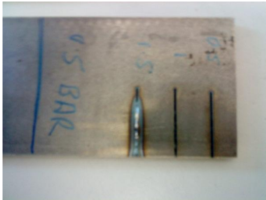
Figure 1 : cut for 0.5 bar pressure
